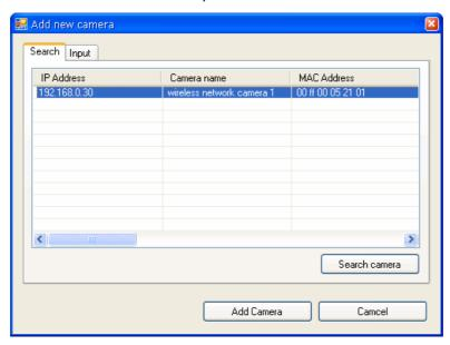
Select the Input tab to add a camera by entering its IP address directly. Enter the camera's IP address (default: 192.168.0.30) and Port (default: 80), and then click Add Camera.
